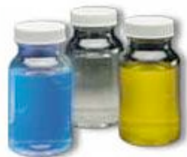
The IDEXX Colilert Test www.idexx.com (yellow total coliform +, fluoresce E. coli +)
