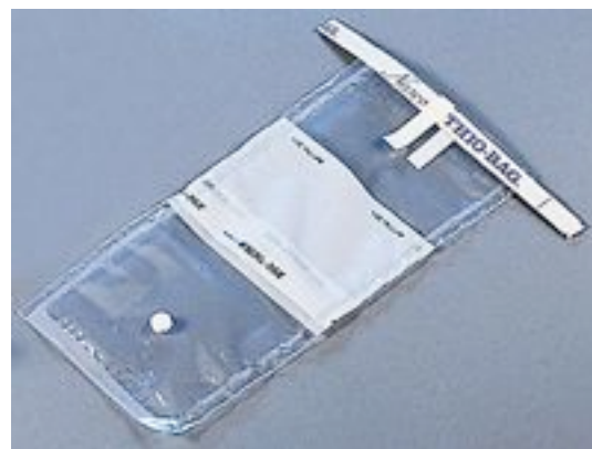
A WhirlPak™ sample collection bag (with a thiosulfate tablet to inactivate any chlorine present) www.hach.com
